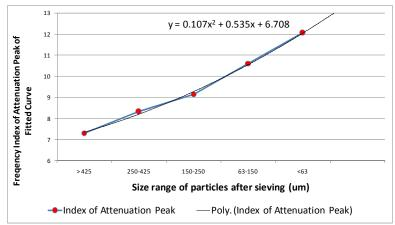
Figure 5 Measured frequency shift of the attenuation peak for changes in mean slurry particle size
