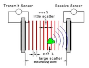
Figure 2 Illustration of ultrasonic attenuation by a particle located between two transducers.
