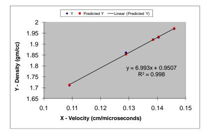
Figure 8 Relationship between Ultrasonic Velocity and Density.
