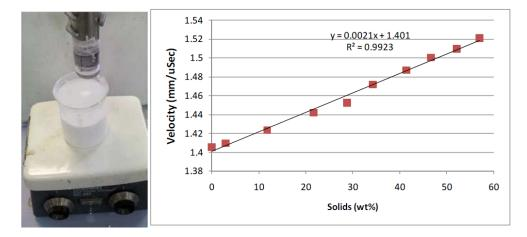
Figure 6 This graph illustrates the relationship between amount of drying of an explosive and ultrasound velocity through the explosive.
