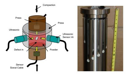
Figure 7 a.) Ultrasound Press Analyzer Concept (left) b.) Ultrasound Instrumented Die (right)
