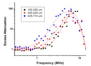
Figure 4 Measured ultrasonic attenuation for three slurries with different particle size ranges
